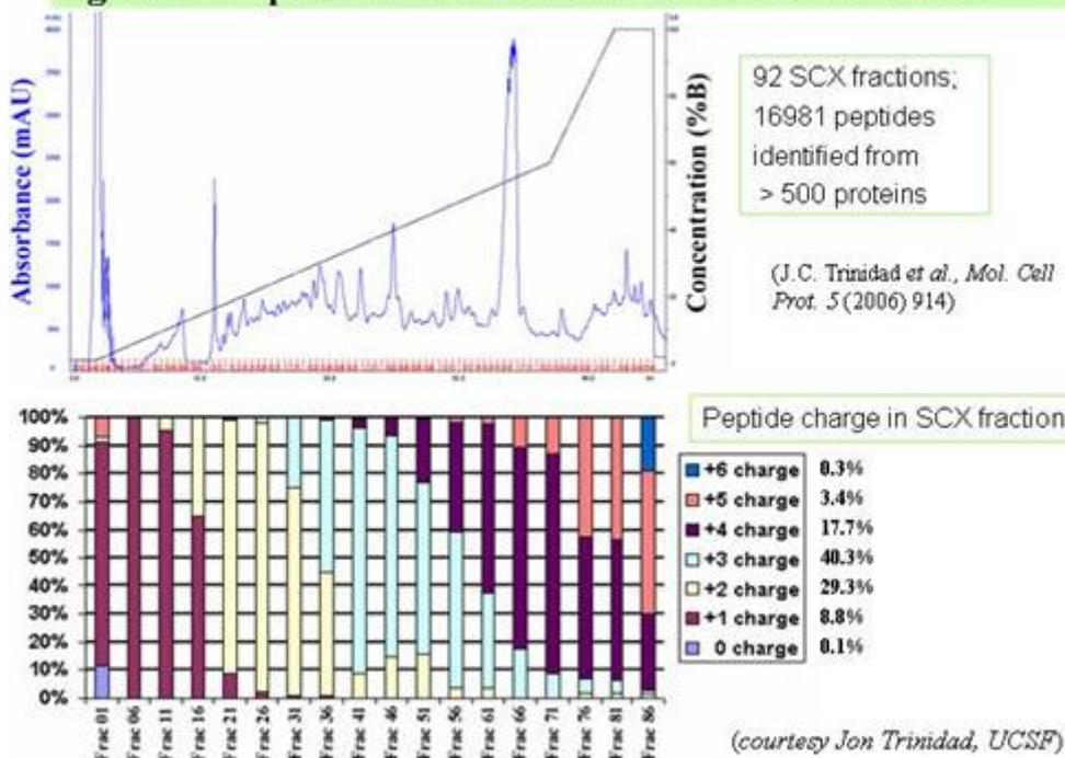
Online vs. Offline SCX Fractionation: Packed capillaries of **PolySULFOETHYL A™** can be eluted via steps of increasing salt concentration, with each fraction going to a desalting RPC trap cartridge or directly to a RPC capillary. This arrangement is commonly called **MuDPIT**. The alternative is to collect fractions offline and then inject them separately onto the RPC capillary ("**divorced MuDPIT**").
